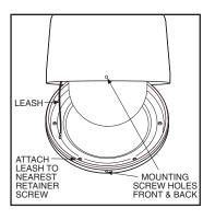
b. Attach the back box trim leash to the lower dome. Use the retainer screw (nearest to a mounting screw) inside lower dome.
